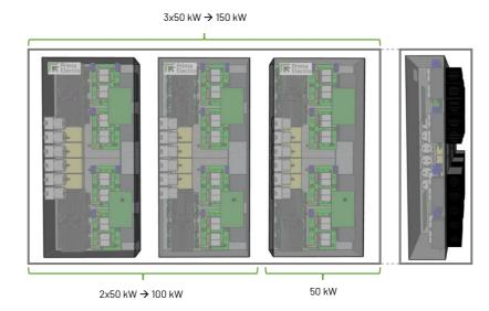
Example of 150 kW DC charging point with 3x50 kW modules
